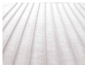
Figure 11: Imprinted lines shaped by the extrusion profile of the 3D-printers nozzle by Mirja Kreuziger.
